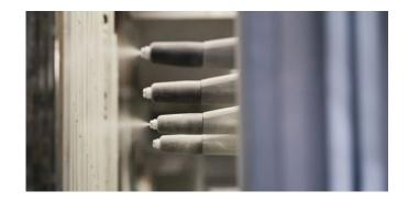
Metal factory's paint lines use powder paints, which is one of the most popular surface treatment methods in the metal industry. Powder paints do not contain solvents or heavy metals and are therefore environmentally friendly. Any leftover paint from the paint lines is collected and recycled.
